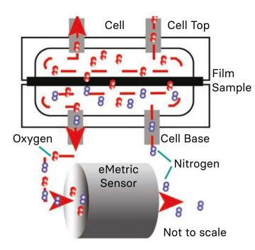
Systech Illinois' eMetric sensor analyzes 100% of the oxygen passing through the sensor resulting in unequivocal conformation of ASTM D3985.
