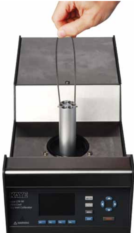
Block Design with two reference holes (I/RTD) and four T/C holes (three T/C/hole).
